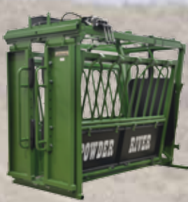
HC2000 Hydraulic Curtain Style Chute
